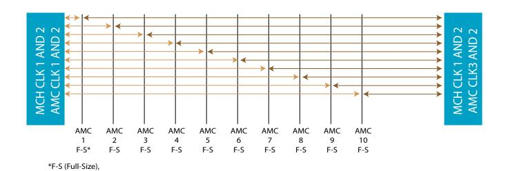
FIGURE 6. VT862 redundant clock Topology
