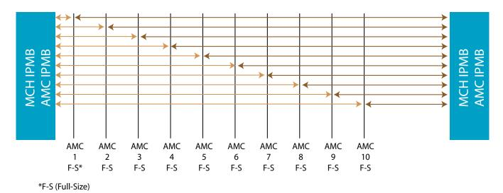
FIGURE 1. VT862 Topology for AMC I2C Bus
