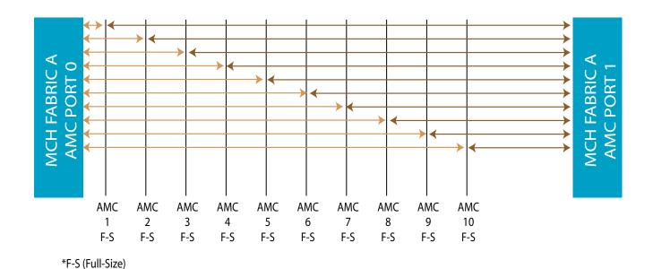
FIGURE 2. VT862 Topology for AMC Ports 0 and 1
