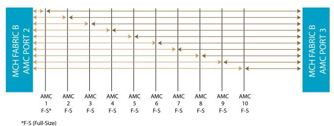
FIGURE 3. VT862 Topology for AMC Ports 2 and 3
